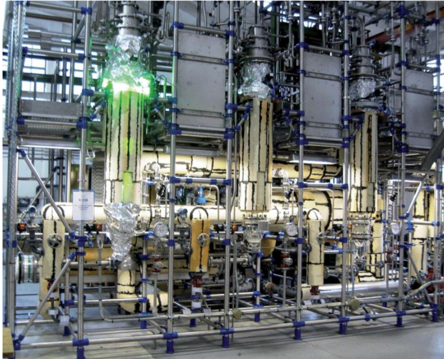
Industrial photoreactor operated by Sanofi (synthesis of artemisinin)
