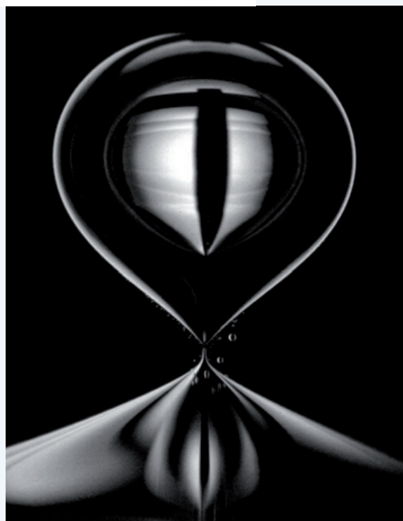
"In the privacy of a border crossing": air bubble that passes through an interface between water and oil. LAGARDE Antoine, doctoral student in fluid mechanism (Paris).
