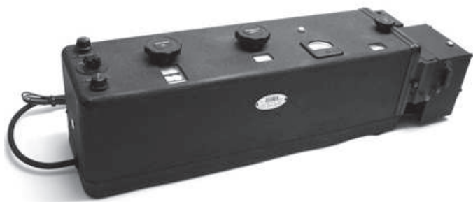
Figure 2 - Spectrophotometer in the DU range designed and manufactured by Beckman Instruments, 1940s. An early example of the "black box". Collection of the National Museum of American History, Smithsonian Institution, Washington DC.
