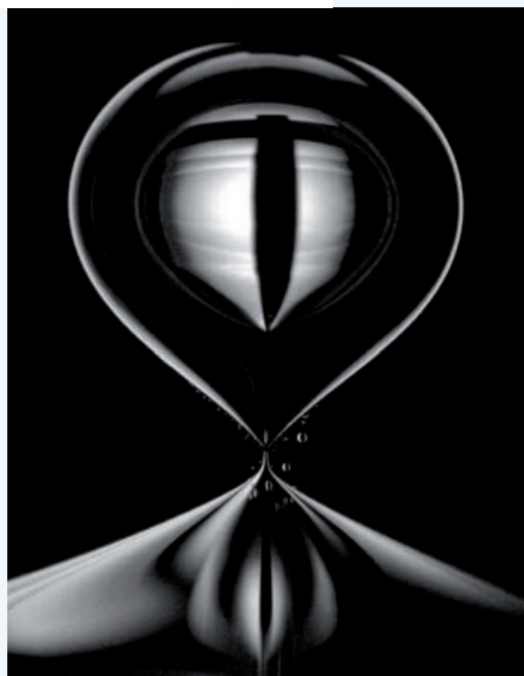
"In the privacy of a border crossing": air bubble that passes through an interface between water and oil. LAGARDE Antoine, doctoral student in fluid mechanics (Paris).
