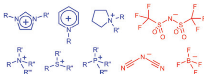
Figure 1 - Representative ionic liquid cations (blue) and anions (red). Top from left: imidazolium ( C_n C_m im^+ ), pyridinium ( C_n py^+ ), pyrrolidinium ( C_n C_m pyr^+ ), bis(trifluoromethylsulfonamide) ( NTf_2^- ). Bottom from left: quaternary ammonium ( N_{nopq}^+ ), tertiary sulfonium ( S_{nop}^+ ), quaternary phosphonium ( P_{nopq}^+ ), dicyanamide ( DCA^- ), tetrafluoroborate ( BF_4^- ). Subscripts m, n, o, p, and q represent the lengths of hydrocarbon side chains. Adapted from [35] with permission from The Royal Society of Chemistry.
