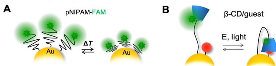
Fig. 1. Fluorescence nano-switches based on thermo-responsive pNIPAM (A) and host/guest interactions sensitive to electrochemical stimuli or light (B).
