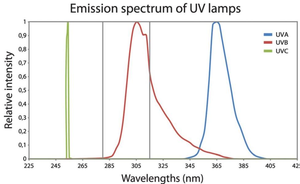
Emission spectrum of the different UV lamps. UVA, UVB and UVC irradiations were performed with B100 (UVP), RPR-3000 (Southern New England Ultraviolet Co.) and BLE-8T254 (Spectronics Corporation) lamps, respectively. The spectra were derived from manufacturer's specifications and modified according to measurements made using an International Light double monochromator spectroradiometer (IL7000/760D/790).
