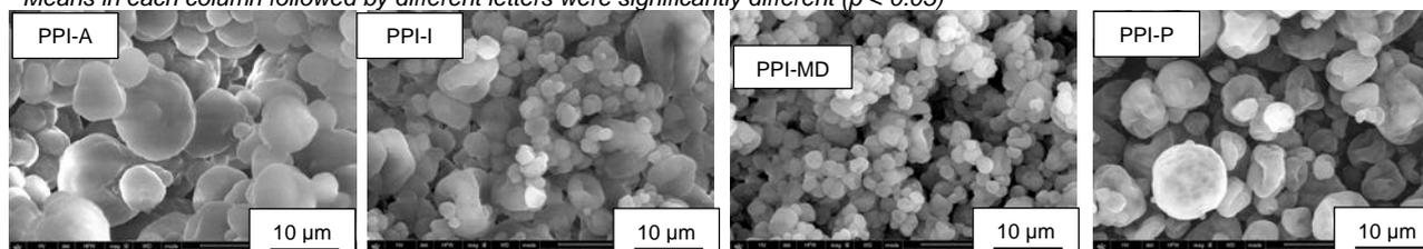
**Figure 1.** Environmental scanning electron micrographs of microencapsulated sunflower oil in pea protein isolates and alginate (PPI-A), pea protein isolates and inulin (PPI-I), pea protein isolates and maltodextrin (PPI-MD) and pea protein isolates and pectin (PPI-P). The magnification was set at 2500x.
