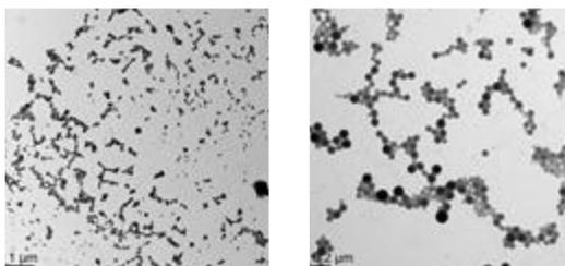
Figure 2. TEM images of aqueous dispersions of iodinated polymer before (left) and after centrifugation/redispersion.
