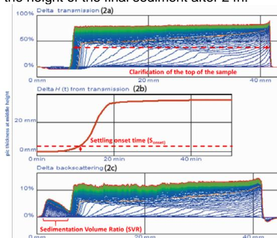
Figure 1: Typical transmission profile (top), backscattering (bottom), peak thickness (middle).
