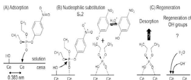
Fig. 1. Degradation mechanism of Paraoxon
