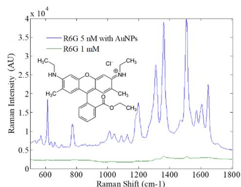
**Fig. 1.** Rhodamine 6G Raman signal enhancement by AuNPs
