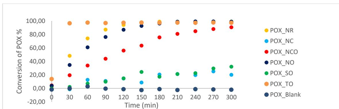
Fig. 2. Degradation efficiency of Paraoxon with different morphologies of CeO<sub>2</sub>
