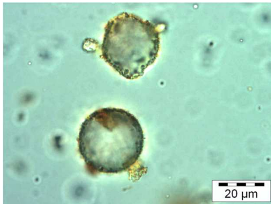
Example of an emulsion stabilized by a vegetal powder
