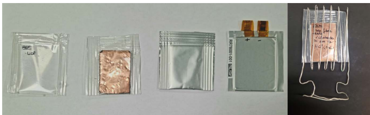
Figure 1 : On left side four of the different pouch studied. The first one is full of LiCl, the second and the third ones contains both two electrodes of silicon deposited on copper and filled with LiCl. The last one is the industrial cell. On the right the coil used for our experiments.
