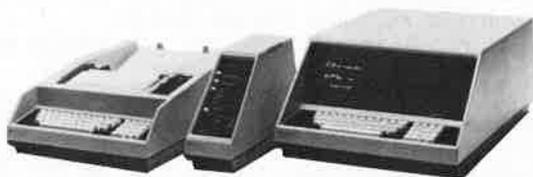
The chromatographer's data system, fully pre-programmed, modular configuration consisting of up to 16 data stations, printer plotters, remote terminals, a central processor and floppy disc storage.
