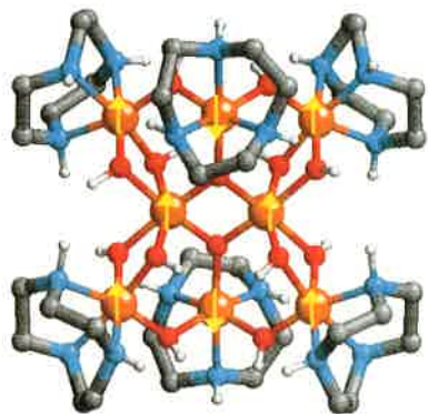
Figure 5 - Structure of Fe 8 . The arrows indicate the preferred spin orientation in the ground state.
