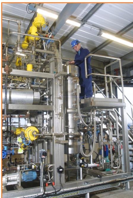
Figure 4 - View of the reactors in the Thomas Swan and Co. Ltd. scCO<sub>2</sub> plant in Consett, Co. Durham (UK).
