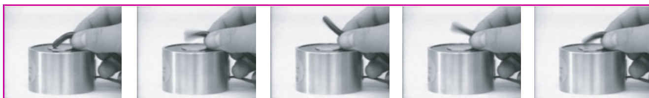
Figure 10 - Snapshot of shape change of a magnetite loaded polyvinyl alcohol hydrogel due to modulated magnetic field. The frequency of the field is 40 Hz.
