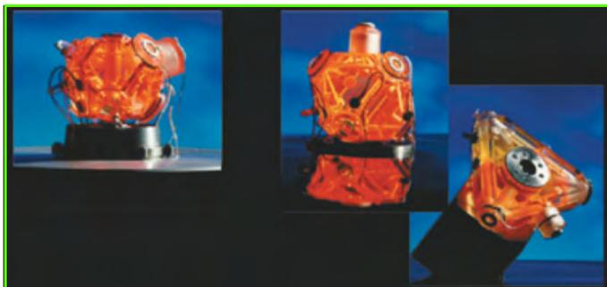
Figure 3 - Gyroscopes lasers Thalès.
