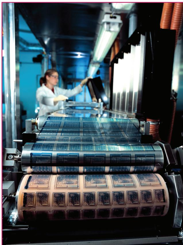
Figure 3 - Fabrication roll-to-roll. © PolyIC press picture.
