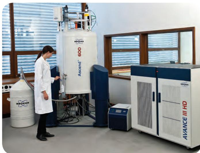
600 MHz NMR spectrometer with CryoProbe Prodigy and SampleMail™ sample transfer system.
