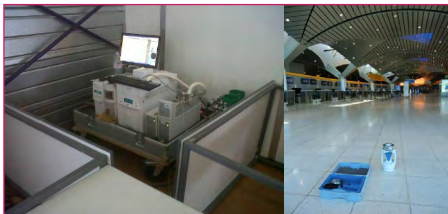
Figure 12 - Gas analysis (© Explorair) and microbiological sampling (© Nosoco.Tech) in Saint-Exupéry Airport (Lyon, France).
