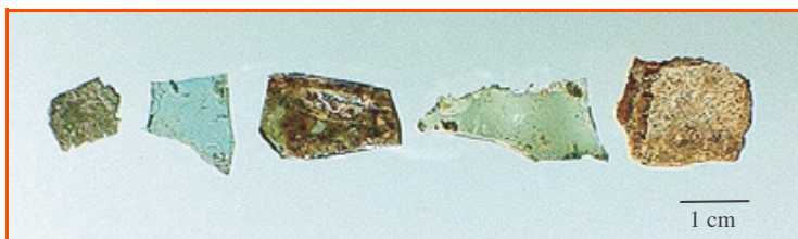
Figure 3 - Selection of archaeological glass fragments with various phenomena of decay.
