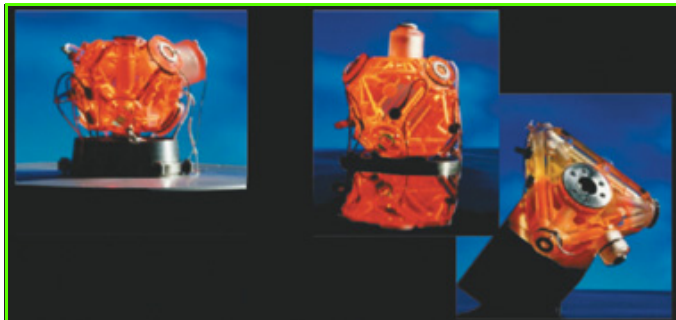
Figure 3 - Gyroscopes lasers Thalès.
