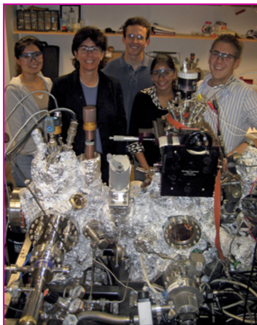
Professor Cynthia Friend and several members of her research group in the laboratory with a scanning tunneling microscope system used for imaging surfaces at the atomic scale, covered with aluminum foil. From left to right: Ms. Xiaoying Liu, Chemistry graduate student, Prof. Friend, Mr. Ryan Quiller and Dr. Dilini Pinnaduwaage, recent doctoral recipient in Applied Physics, and Mr. Thomas Baker, Chemistry graduate student. (The photo was taken by Dr. Weiwei Gao, a postdoctoral fellow in the group and an accomplished photographer).
