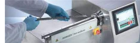
Thermo Fisher Process 11 (D = 11.0 mm et L/D=40.0), max 10g/min
