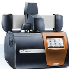
Differential Scanning Calorimeters
