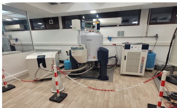
Figure 1: Ascend EVO 600 MHz AVANCE NEO with a QCI cryoprobe
